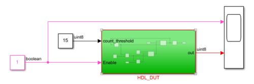
Add your design targeted for ASIC/FPGA inside HDL\_DUT and then run the following command: makehdl('HDL\_DUT')
