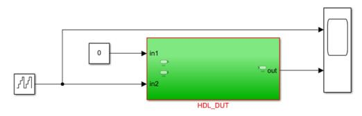
Add your design targeted for ASIC/FPGA inside HDL\_DUT and then run the following command: makehdl('HDL\_DUT') The **Blank DUT** template has a HDL\_DUT subsystem that corresponds to the Design-Under-Test (DUT) for which you generate HDL code. To verify the DUT functionality, the template contains a test bench outside the HDL\_DUT subsystem that provides inputs to the DUT and logs output values. See "Partition Model into DUT and Test Bench".
