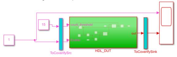
Add your design targeted for ASIC/FPGA inside HDL\_DUT and then run the following command:
