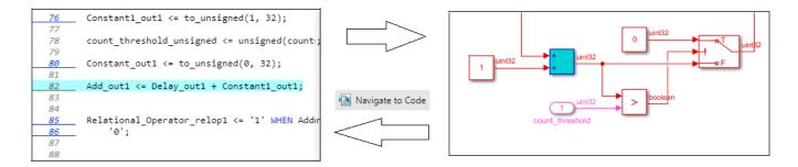
See "Navigate Between Simulink Model and HDL Code by Using Traceability" and "Create and Use Code Generation Reports".
