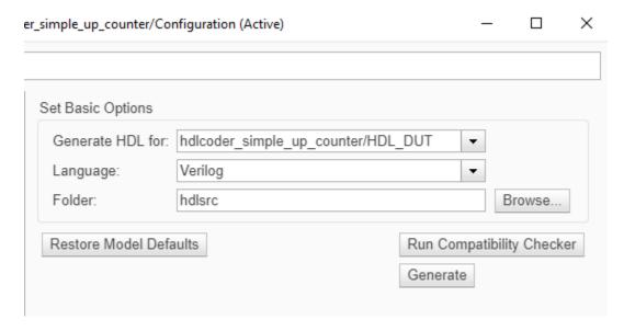
HDL Coder compiles the model and generates the test bench.
