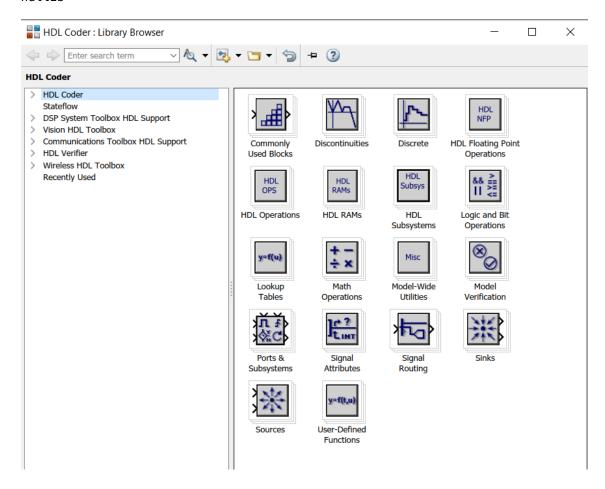
Blocks in the **HDL Coder** Library are available with Simulink. If you do not have HDL Coder, you can simulate the blocks in your model, but cannot generate HDL code.
