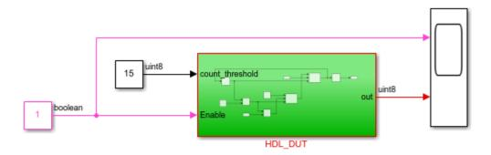
Add your design targeted for ASIC/FPGA inside HDL\_DUT and then run the following command: makehdl('HDL\_DUT')
